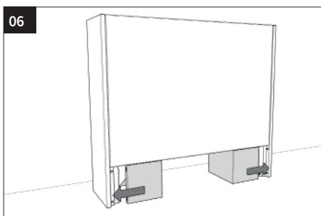
Slide the pedestals under the casing and push them in the mounting holes (click system).
