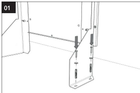
Drill holes in the floor and fix with the correct mounting material. Place the device at least 10 cm from a wall. Otherwise you will not be able to place the mounting screws..
