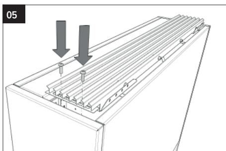
Mount the grille with the screws, 2x left and 2x right
