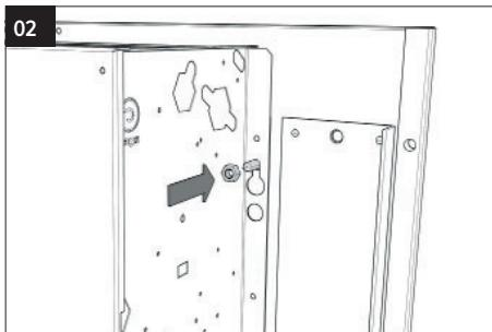
Push the flat bolts through the back panel to the front, hook the device. Put the nut on the bolt and tighten.
